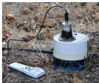
Fig. 1: Measuring CO 2 -Fluxes from the soil. Photo: L. Munjonji
